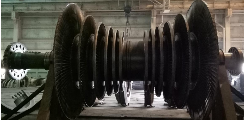
Figure2.2: Turbine of Barapukuria 125 MW unit
