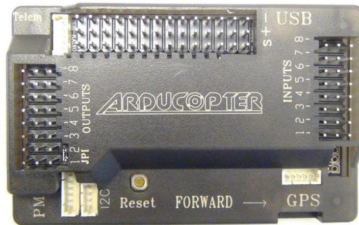
Figure 2.2 : APM 2.8 Flight Controller [8]
