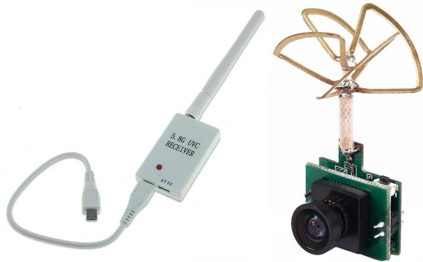
Figure 2.11 : FPV Camera transmitter and receiver [17]
