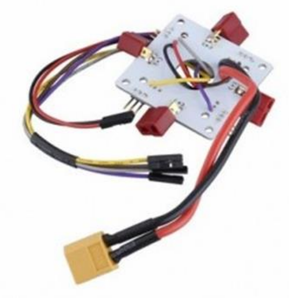
Figure 2.8 : Power Distribution Board [14]
