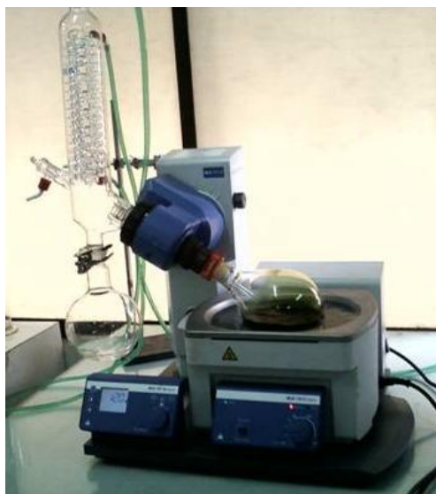
Figure 3.1.5: Drying of extract using rotary evaporator.
