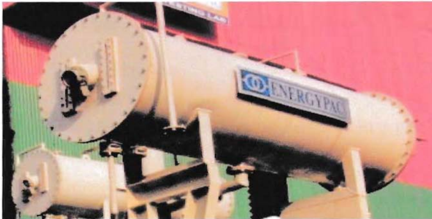
Figure -: Conservator Tank of a transformer
