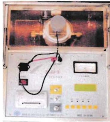
Figure -: An example of Oil Tester used at Energypac
