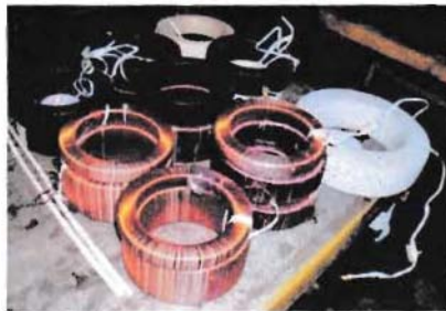
Figure -: Protection coil; metering coil
