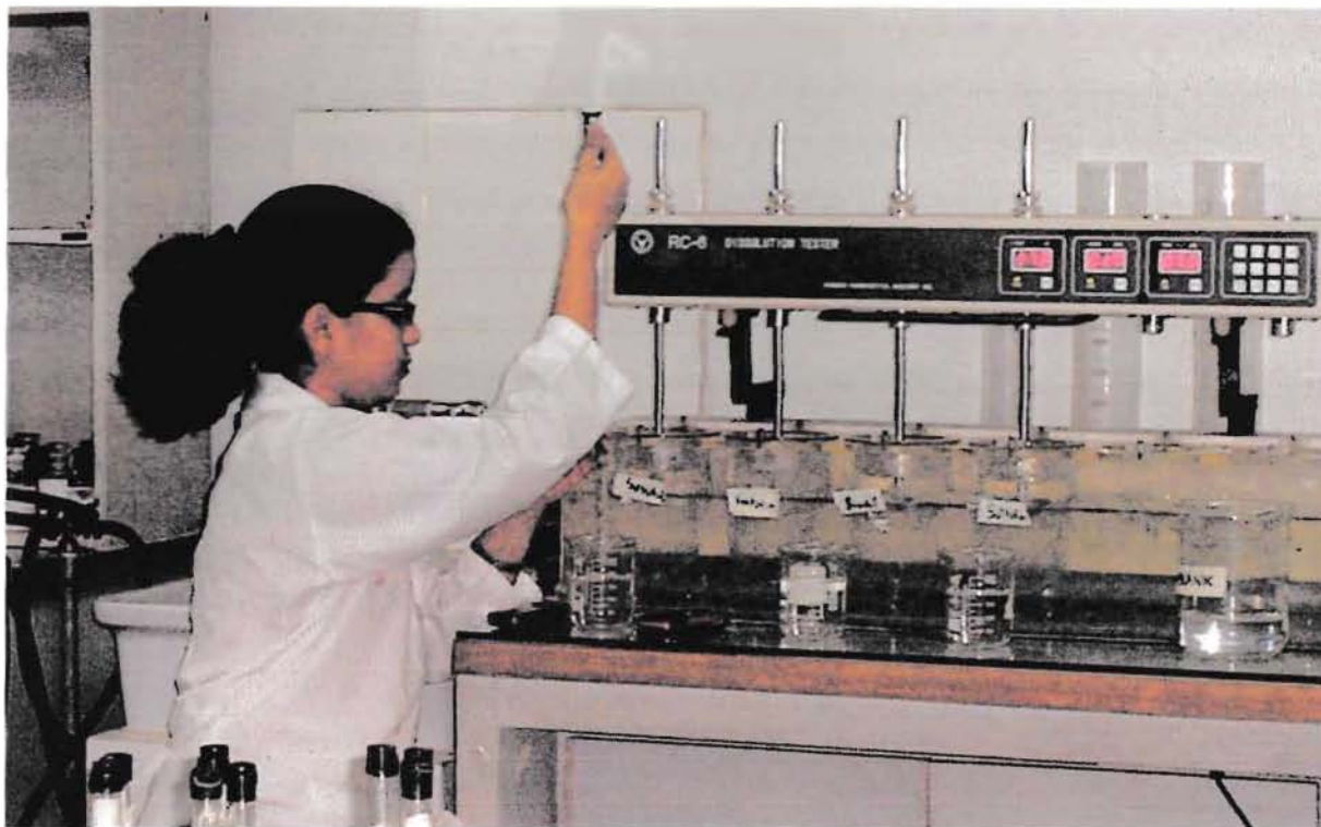
Figure 12. Working with the dissolution tester while the 120 minutes running time was continuing.
