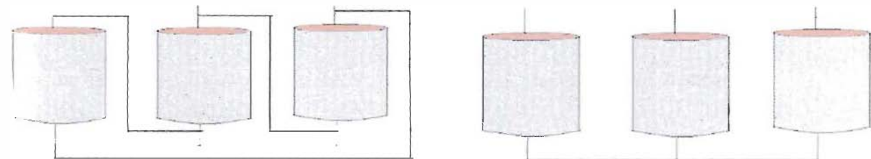
Figure 10: Delta connection (left) and Y-Connection (right)
