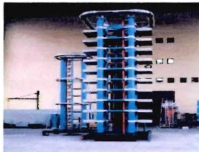
**Fig 18: Impulse Voltage Test System. [6]**
