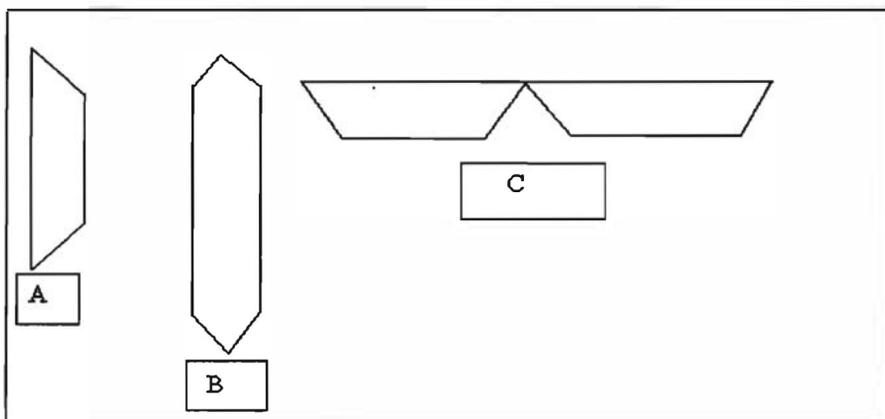
**Fig 6: Transformer Core Shape. [2]**
