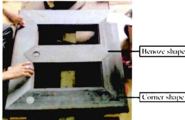
**Fig 9: Core Assembling. [3]**
