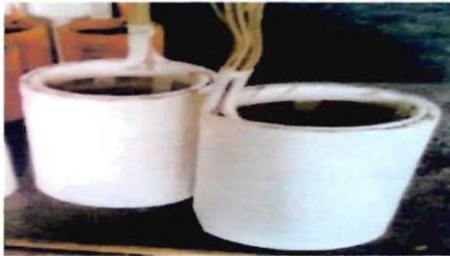
**Fig 3: Low Voltage Coil. [1]**
