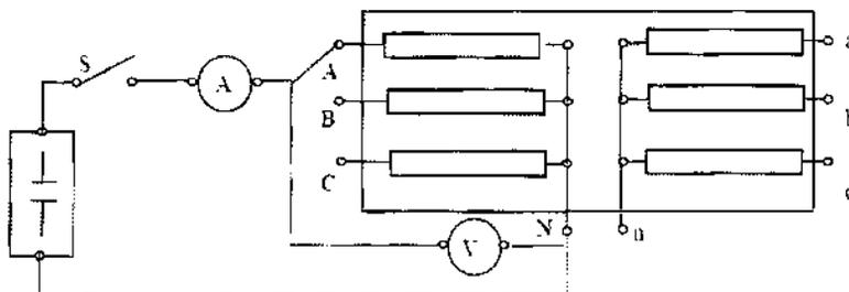
**Fig 15: Circuit Diagram of Winding Resistance Measurement.**
