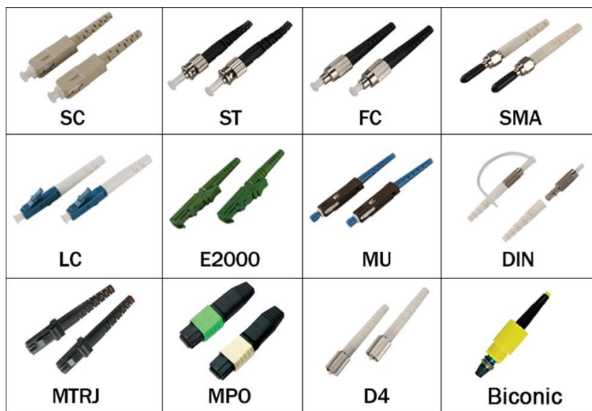
Figure: Different types of connectors
