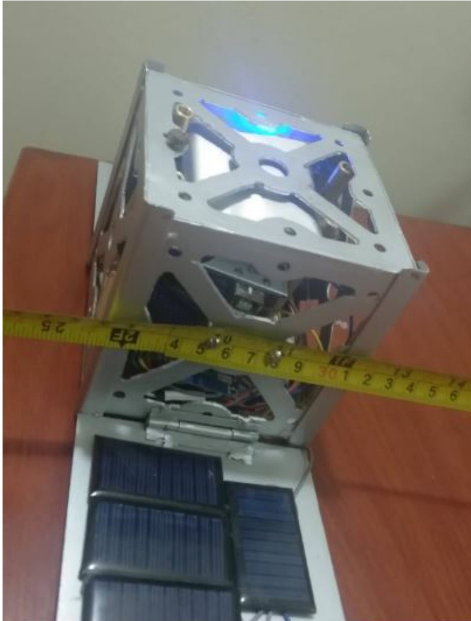
Figure 6.1: Making Monopole antenna by measuring tape
