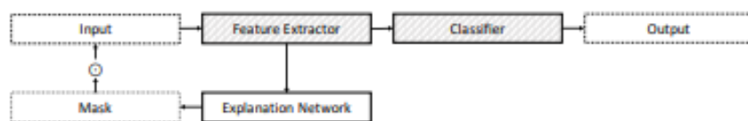
Fig. 4.7. Architecture of the explanation mask. The pre-trained (top) network is divided into a component to extract and classify features. The function extractor output feeds into an explanation network, generating a mask multiplied with the input element-wise. The masked input is supplied to the final output through the initial network. Shading shows weights that are frozen.
