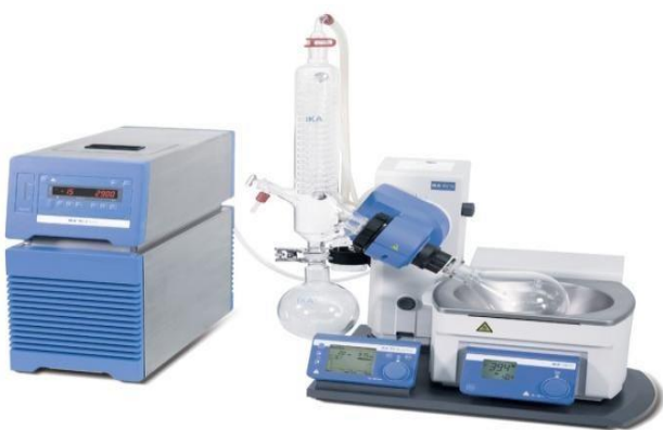
Figure 3.1: Drying of extract using rotary evaporator
