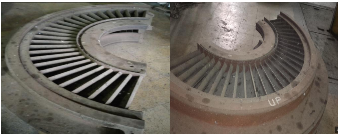
Figure 4.4: Fixed blades of turbine.
