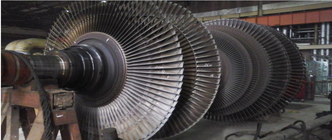
Figure 4.3: Moving blades of low pressure cylinder.
