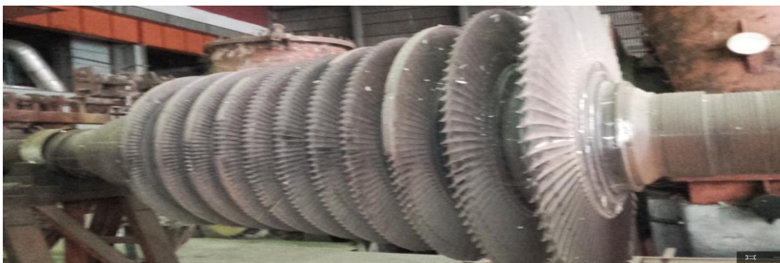
Figure 4.2: Moving blades of intermediate pressure cylinder.
