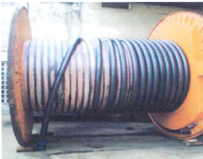
Figure 5.13: Underground cables at APSCL for 132KV line.
