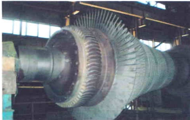
Figure 2.5: Picture of Impulse Turbine of APSCL unit 3 (150MW)
