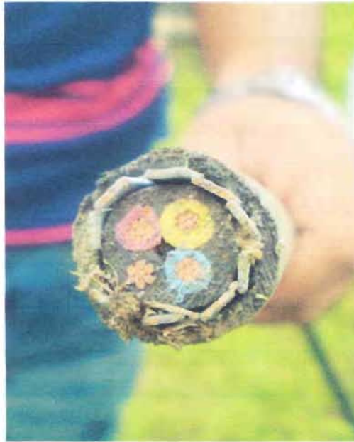
Figure 5.15: Cross section of High Tension Cable
