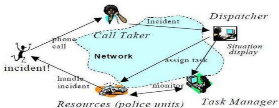
Figure 3.1 : Basic operational scenario in a CAD system for police
