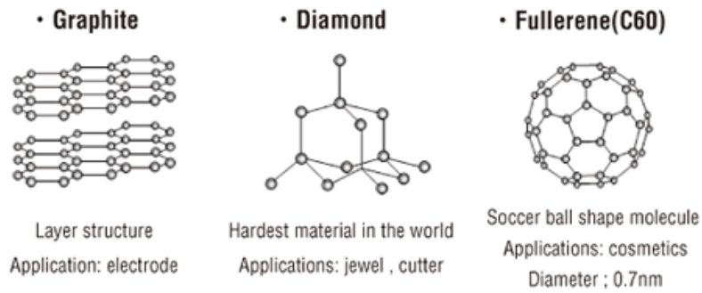
Figure.1.1 Structure of Graphite, Diamond and Fullerene
