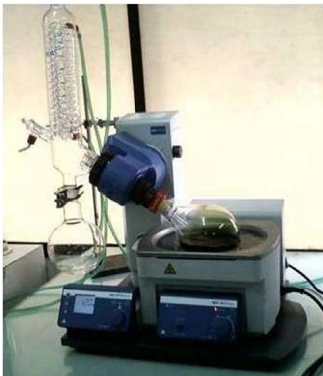
**Figure 3.1:** Drying of extract using rotary evaporator
