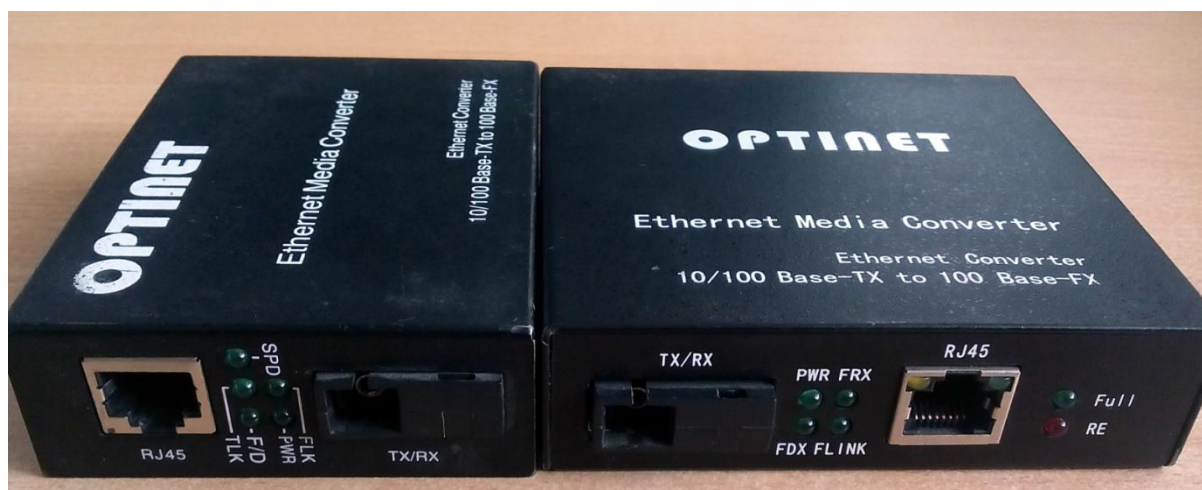
Figure: 6 – Media Converter [Captured during practical work]
