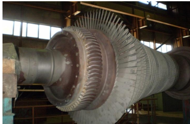
Figure 4.1: Impulse steam turbine of APSCL [5].
