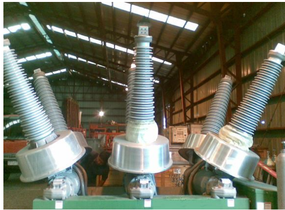
Figure 6.3: SF6 circuit breaker with normal current rating is 1250 A
