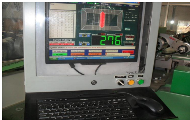
Figure 6: Computerized core cutting machine
