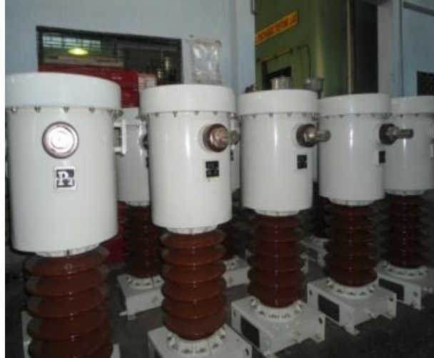
Figure 21 : Outdoor Current Transformer
