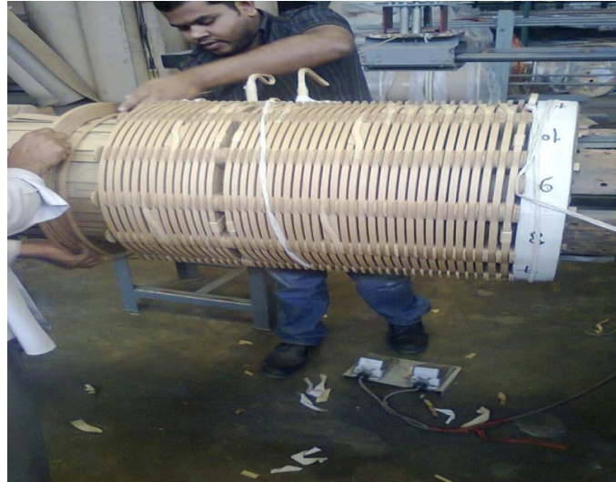
Figure 3: Coil winding (using coil winding machine)
