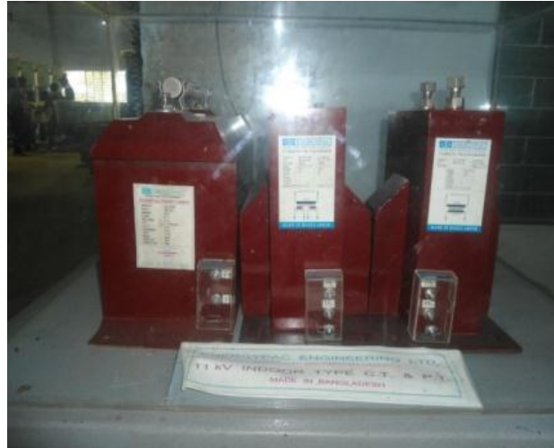
Figure 24 : 11kV Indoor Type CT & PT
