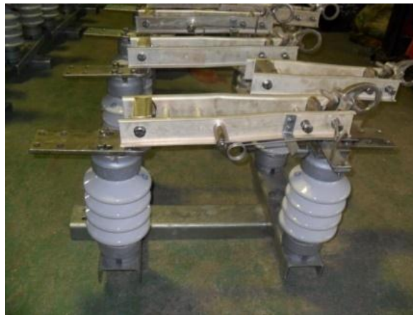
Figure 31 : Auto Voltage Regulator Switches
