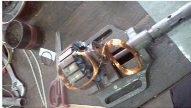
Figure 4.7: Motor winding and repair section.
