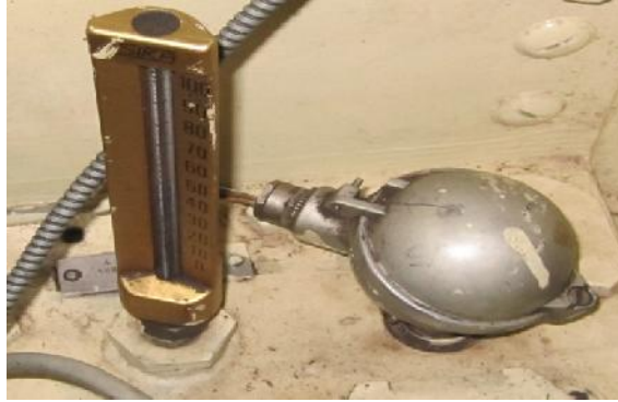
Figure 4.10: Thermocouple for measure shaft temperature.
