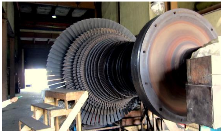
Figure 2.6: LP turbine used in 150 MW & 15.75 KV of APSCL.
