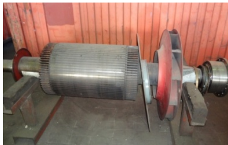
Figure 2:3: AC Generator Rotor in unit-5
