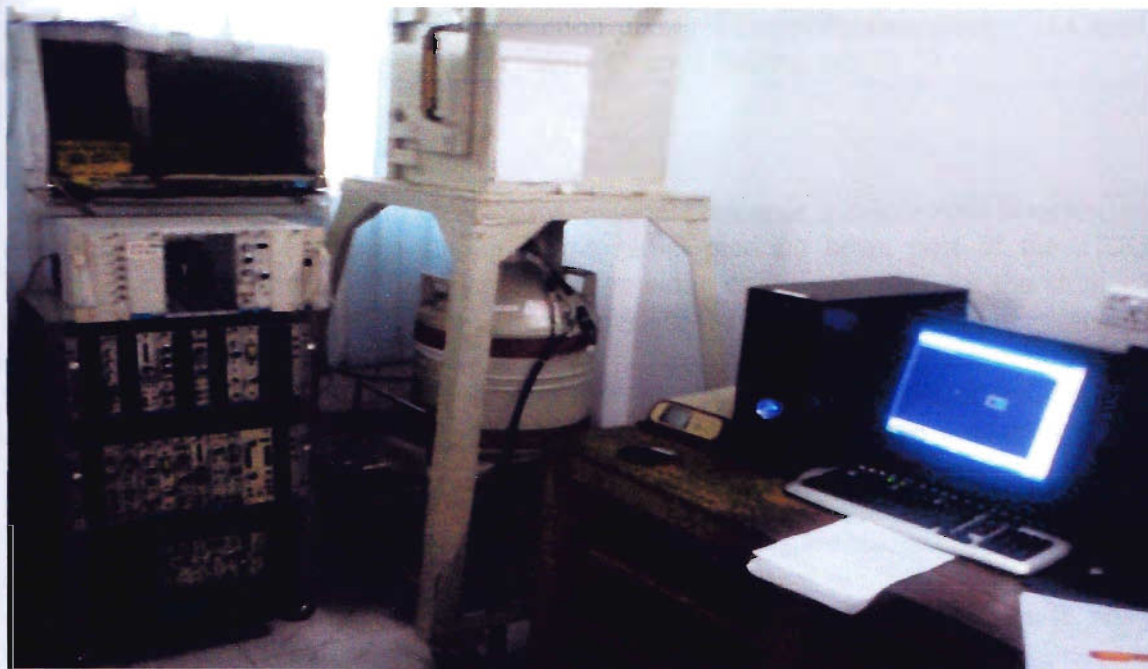
FIG 1.2: HPGe Detector with MCA in BAEC
