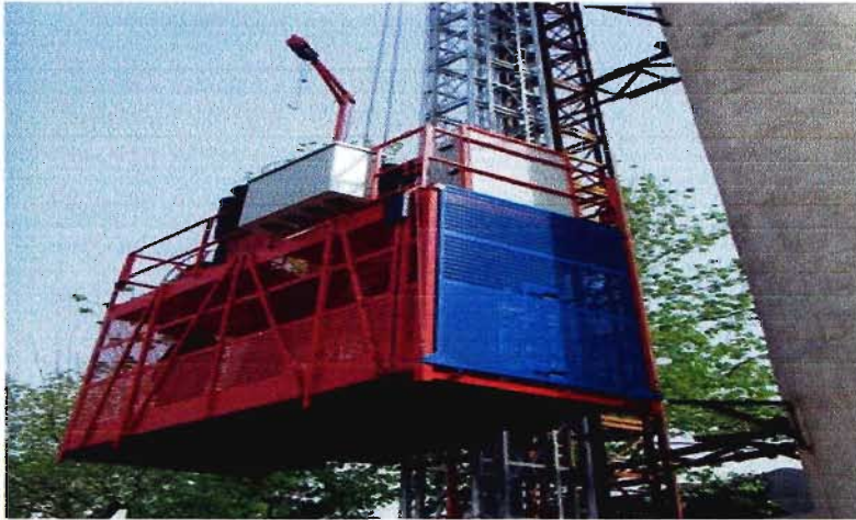
Figure 18: Conventional Cargo Lift
